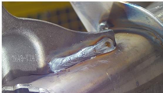
Figure G.2: Example of an OK welding image from cordon c19 in Renault Welding dataset.
